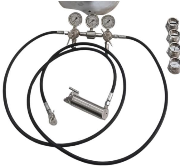
Nitrogen regulator panel, hoses and reverse-exhaust cylinder
