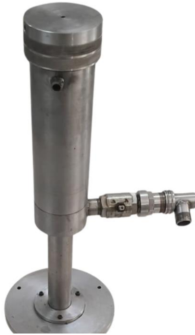
Lost Circulation Material (LCM) Tester, IM-LCM-TER07
