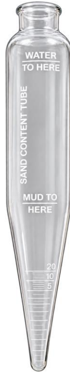
Graduated sand content tube, showing the “Water to Here” and “Mud to Here” fill marks
