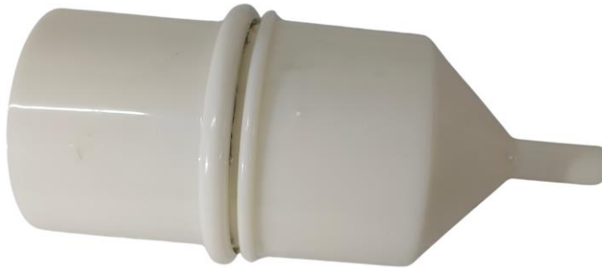
Funnel — directs washed sand cleanly from the sieve into the graduated tube
