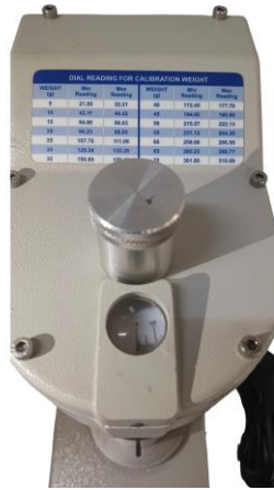
Factory calibration-weight table, printed on the instrument head
