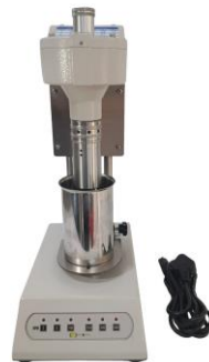
The IM-RV-D6 head, rotor and bob assembly, mounted on its support column and base
