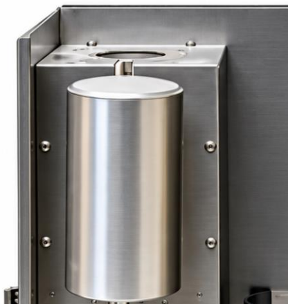
Fig. 2 — The heating chamber's insulated cover and insertion port, which receives the assembled distillation/condensation body
