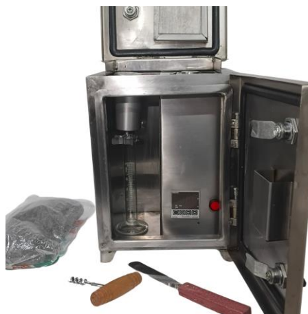
Cabinet interior, front door open — graduated receiver, digital temperature controller, and door-mounted accessory pocket, with steel wool, spatula, and corkscrew tool
