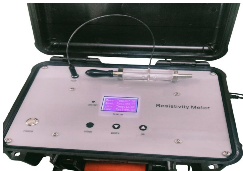
The LCD display shows measured and temperature-converted readings together — shown here mid-test with the resistance cell and temperature sensor connected
