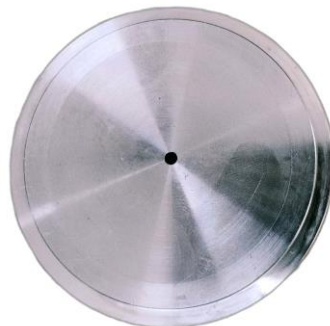
Lid with center vent hole — fluid weeps out here as it seats fully home
