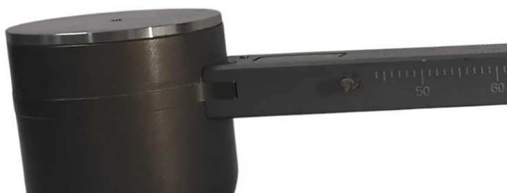
Rider and graduated beam at the cup end — read from the scale edge closest to the cup
