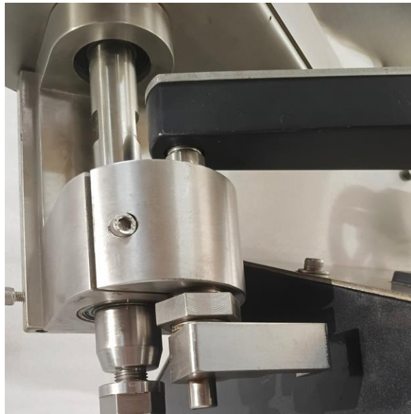
Close-up of the shaft and pivot assembly where the ring and block mount
