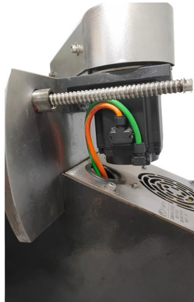
Motor and lead-screw assembly at the base of the stand
