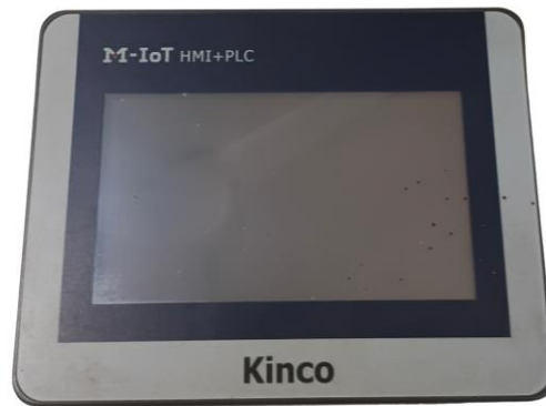
Touchscreen HMI + PLC control panel
