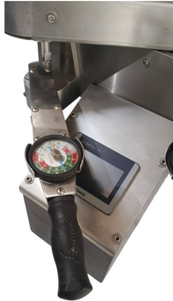
Calibrated torque wrench mounted on the torque arm
