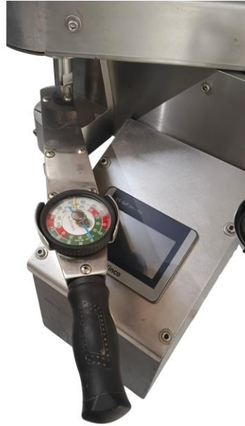
Torque wrench being adjusted during the coefficient-of-friction test
