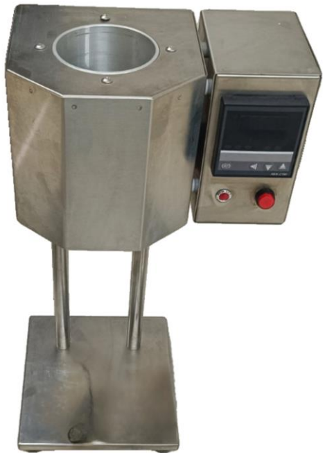
The IM-FP-HTHP175 heating jacket, cell and pipe-manifold assembly, mounted on its base
